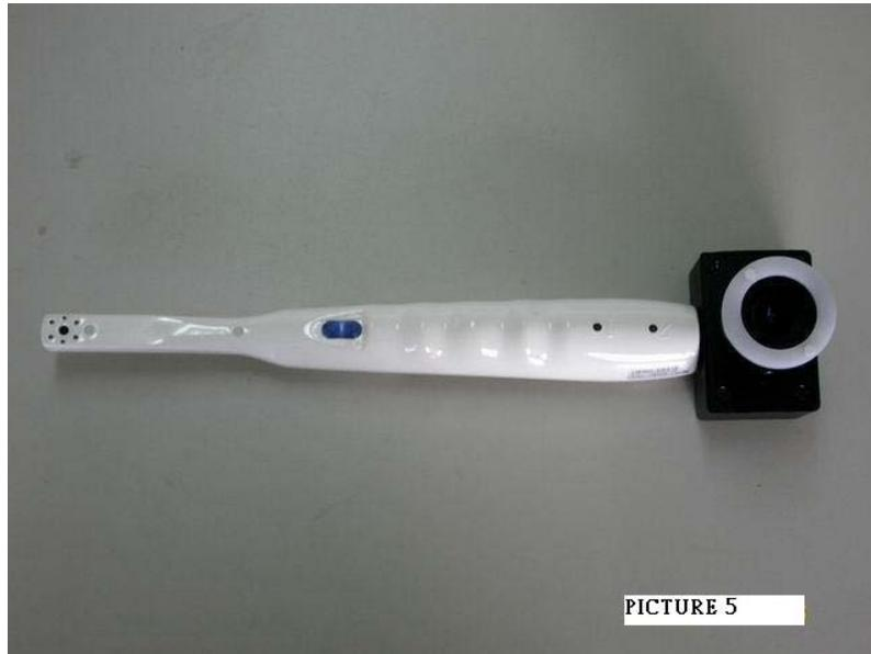
Plug the Extraoral Camera to the bottom of Discovery wireless intraoral camera handpiece. Be sure to plug Extraoral camera in right direction. ( refer to Picture 4 and Picture 5 ).
