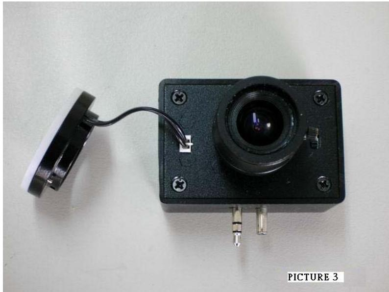
Connect diffuser light according to Picture 3.
