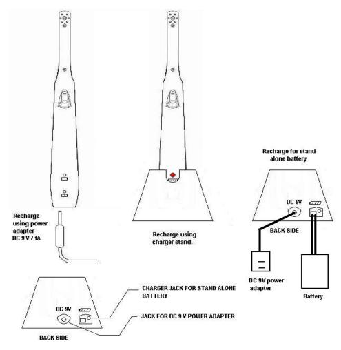
When the battery is fully charged, the RED LED will turn off.
